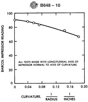
FIG. X1.1 Effect of Curvature of Sheet on Barcol Impressor Readings-Model 934-1, 0.064-in. thick 2024-T3
