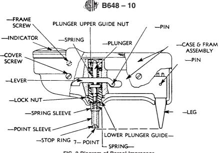
FIG. 2 Diagram of Barcol Impressor
