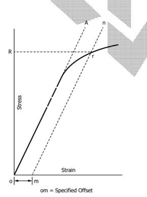
FIG. 9 Stress-Strain Diagram for Determination of Yield Strength by Offset Method
