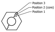
FIG. A3.7 Hardness Test Locations
