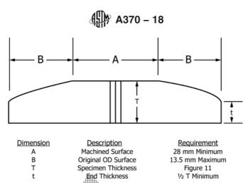
FIG. 12 Tubular Impact Specimen Containing Original OD Surface
