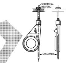
FIG. A4.2 Snubbing-Type Gripping Device
