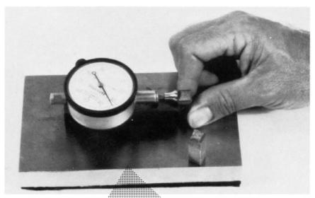
FIG. 16 Lateral Expansion Gauge for Charpy Impact Specimens
