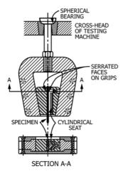
FIG. A4.1 Wedge-Type Gripping Device
